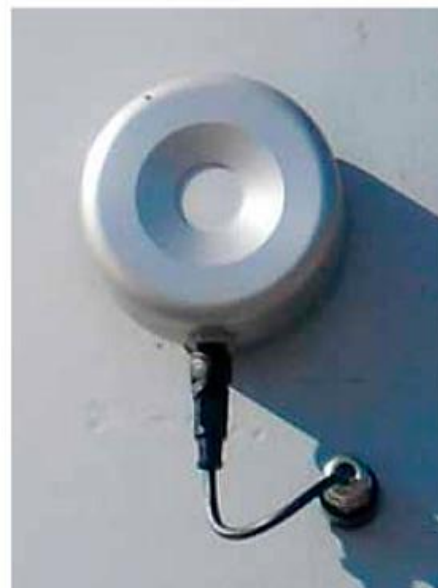
The sensors are magnetised for cost-effective installation.
